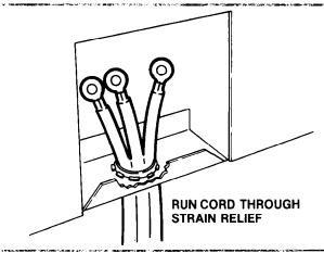
Run cord or cable through strain relief.
