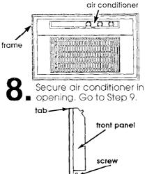
**9** Remove sheet metal screws from front base flange. Insert tabs on the top edge of front panel into slots in the air conditioner cabinet. Use two screws to attach the bottom of the front panel to the cabinet.
