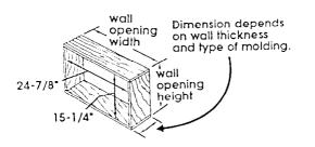
2 Cut opening through the wall. Remove insulation.
