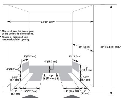
Water line should enter through the left side of opening in shaded areas. Minimum 1/2" (12,7 mm) hole. Power supply line should enter through the right side of opening in shaded area Power sunnly line hole-direct wired: 3/4" (1.9 cm) Power supply line hole-with plug: 1-1/2" (3.8 cm)
