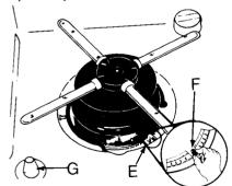
Overflow Protection Float—The blue float (G) in the front left corner of the dishwasher tank prevents the dishwasher from overflowing. The float must be in place for the dishwasher to operate.
