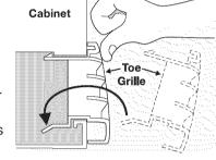
Starting from left side of toe grille, press in on first top tab using your thumb and push toe grille forward until it snaps in place. Continue this process until all tabs are snapped in place and toe grille is secured to refrigerator.
