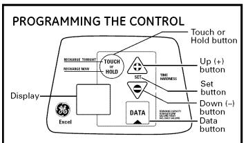
**TIMER SETTINGS REQUIRED** upon installation and after an extended power outage.
