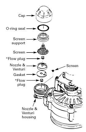
**IMPORTANT:** Be sure small holes in the gasket are centered directly over the small holes in the nozzle and venturi housing.
