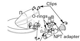
O-ring seal goes into the outer groove only. The clip snaps into the inner groove (see below).
