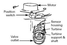
If you don't get a reading in the display, with faucet open, pull the sensor from the valve outlet port. Pass a small magnet back and forth in front of the sensor. You should get a reading in the display. If you get a reading, shut off water supply, unhook the in and out plumbing and check the turbine for binding.
