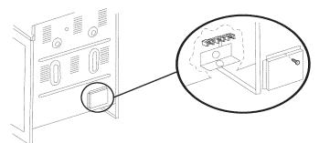
**3.** Remove plastic tag holding three 10-32 hex nuts from the middle post of the terminal block.
