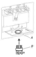
A. Removable retaining nut B. Strain relief
