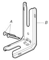
A. #12 x 15/8" screws B. Anti-tip bracket
