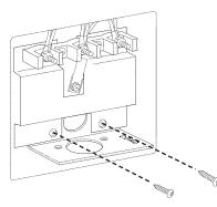
Position cord/conduit plate as shown in the following illustration.
