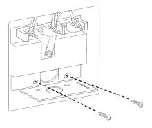
Assemble a UL listed conduit connector in the opening.
