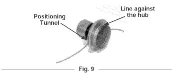
Correctly installed line will be the same length on both sides.
