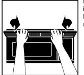
Push the bottom until it snaps into place. Replace the mounting screws.
