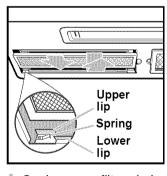
of each filter away from you. This will slide the front of the filter off the lower lip. Swing the front of the filter down and slide the filter out.
