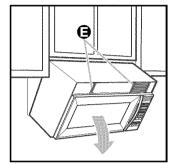
supports **(a)** and firmly pull the microwave oven forward and downward to release the microwave oven cabinet from the mounting plate locking pins **(b)**.
