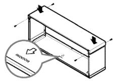
• Assemble the outdoor grille and fasten the 4 screws as shown below.
