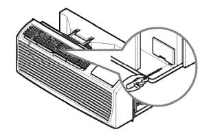
3) Remove the front grille by pulling it out at the bottom to release it, then lift it up along the unit top front.
