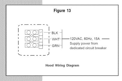
Electrical power source wiring can be connected through the top or back of the hood. Access the wiring inside the hood canopy in the area to the right side of the power ventilator.
