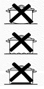
Pans with rounded, curved, ridged or warped bottoms are not recommended. Pan Detection/Sizing may not work properly with these types of pans.
