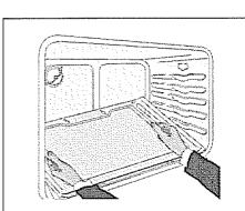
Use the finger openings along the outside edges of the oven bottom to raise and lower the oven bottom.
