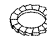
1 safety screw and lock washer, to secure the blower: (screw is marked with red paint)
