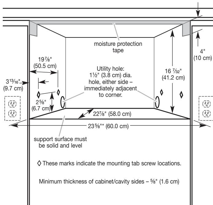
Install the dishwasher in a cabinet cutout that is level, will hold weight up to 104 lbs. (47kg), and is in an area suitable for its size and use.
