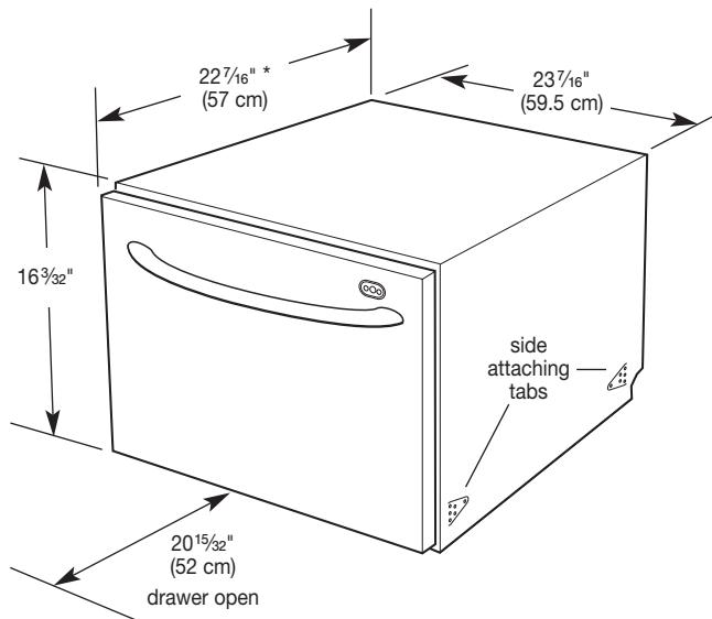
\* If custom wood panels are to be used, the product depth is specified with an  $1\frac{1}{16}$ " (18 mm) door panel thickness.
