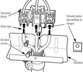
Wire used, location and enclosure of splices, etc., must conform to good wiring practices and local codes.
