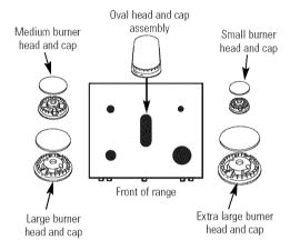
Make sure the slot in the burner head is positioned over the electrode.
