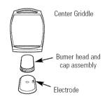
**CAUTION:** Do not operate the burner without all burner parts in place.
