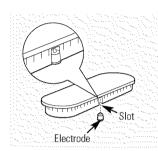
Make sure the slot in the burner head is positioned over the electrode. Use a sewing needle or twist-tie to unclog the small hole in the burner head.
