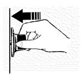
Push in and turn the lower oven drawer knob to any desired setting.
