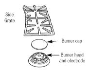
Assemble the center burner. Make sure that the locking feet on the center grate hook over the side grates.
