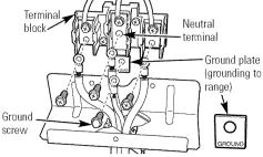
**3** Place the terminal screws and ground screw in safe location for later use.
