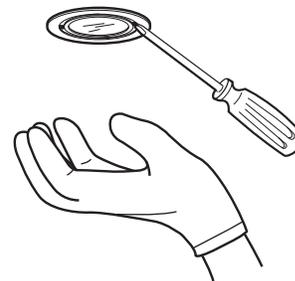
3. Replace with a 12-volt, 20-watt maximum, halogen bulb made for a GU-4 base.
