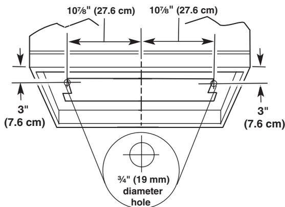
3. Measure and mark lines as shown. Use a saber saw or keyhole saw to cut an opening through the underside of the cabinet.
