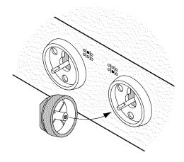
• Put the remaining knobs on the outer valve shafts.
