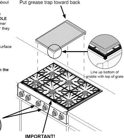
Do not turn burners higher than the **MAX GRIDDLE** setting when using the griddle!
