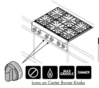
• When installing the knobs, align the "D-shaped" opening on the back of the knob with the end of the valve shaft. Carefully push the knob on until it stops.
