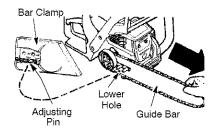
Install bar clamp nuts and finger tighten only. Do not tighten any further at this point.
