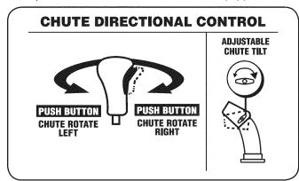
The chute directional control is located on the left side of the dash panel.
