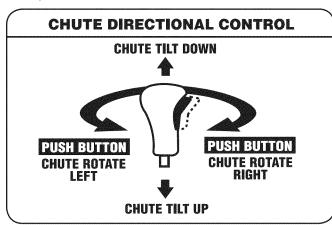
4-Way Chute Directional Control (if so equipped)
