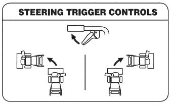
The left and right wheel steering trigger controls are located on the underside of the handles.
