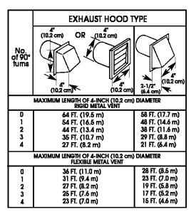
For **exhaust systems** not covered by the exhaust length chart, see <u>Whirlpool Service Manual</u>, "Exhausting Whirlpool Dryers," Part No. 603197, available from your Whirlpool parts distributor.
