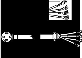
Four-wire power supply cord must have four, No.-10 copper wires and match a four-wire receptacle of NEMA Type 14-30R. The fourth wire (ground conductor) must be identified with a green cover and the neutral conductor by a white cover. **4.** Remove center terminal block screw.
