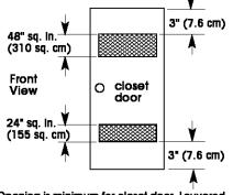
Opening is minimum for closet door. Louvered door with equivalent air openings is acceptable. Companion appliance spacing should be considered.
