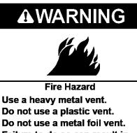
Do not use a metal foil vent. Failure to do so can result in death or fire.
