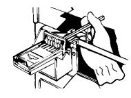
■ Secure coin slide mechanism from inside the control panel using the 3/16" bolt and washer included with the slide mechanism. Install coin box.
