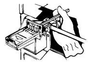
• Secure coin slide mechanism from inside the control panel using the 3/16" bolt and washer included with the slide mechanism. Install coin box.
