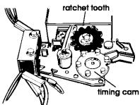
Turn the timing cam by hand until the "V"-shaped notch lines up below the ratchet tooth.
