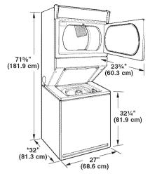
\*Most installations require a minimum 5½" (14 cm) clearance behind the dryer for the exhaust vent with elbow. See "Venting Requirements."
