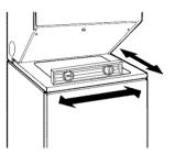
If the washer/dryer is not level, prop up the front with the wood block and adjust the feet up or down as necessary. Remove wood block.
