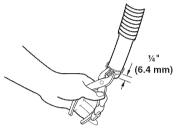
Open clamp. Twist hose back and forth while pushing onto drain connector on the side of the washer/dryer. Continue until hose contacts the ribbed stops on the cabinet.
