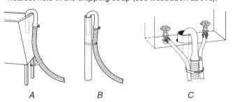
If the water faucets and the drain standpipe are recessed, put the hooked end of the drain hose in the standpipe. Tightly wrap the shipping strap around the water inlet hoses and the drain hose (C above). Push fastener into the nearest hole in the shipping strap (see illustration above).
