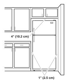
To ensure proper ventilation for your refrigerator, allow for a 1" (2.5 cm) space on each side.
