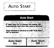
When **"Auto Start On"** is chosen, the washer will automatically start when the cycle is selected.
