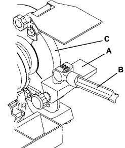
The Wheel Dresser is to be used on the grinding wheel only. It will remove buildup of material on the grinding wheel, remove imperfections and make the corners of the grinding wheel square. See Figure M.
