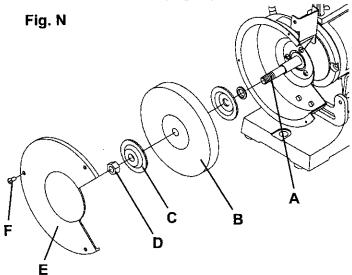
Due to normal wear, both wheels will need to be replaced occasionally. See Figure N.
