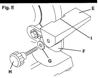
5. Install the Drill Bit Sharpening Plate, by loosening the Right Side Adjustment Knob until there is approximately a 1/4" of threads visible. Place the Plate onto the Right Side Tool Rest and over the visible threads. The Flat Washer must be placed between the Plate and the Adjustment Knob. Tighten the Adjustment Knob.
