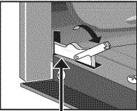
Lock engaged for door removal
