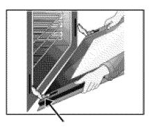
**HINGE SLOT-Door removed** from the appliance
