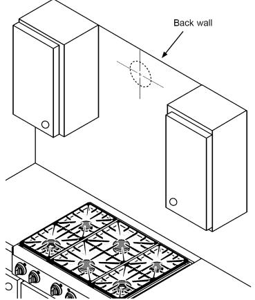
**Duct Cut-Out for Rear Venting**
