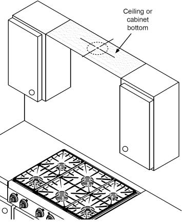
**Duct Cut-Out for Top Venting**
