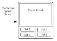
Thermostat will operate on either Set A, Set B or both. When changing, replace with all new batteries. Never use a mix of old and new.
