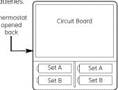
Thermostat will operate on either Set A, Set B or both. When changing, replace with all new batteries. Never use a mix of old and new.
