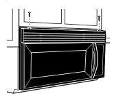
**3.** Tip the grille forward, then lift out to remove.
