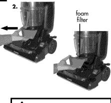
Do not operate vacuum with damp or wet filters, or without all filters in place.
