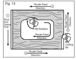
control. This is called "Climb-Cutting:" cutting in the opposite direction of the proper feed direction. "Climb Cutting" increases the chance of loosing control, resulting in possible personal injury. When "Climb Cutting" is required (backing around a corner, for example), exercise extreme caution to maintain control of the router.
