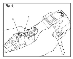
desired cutting depth. The direction of the rotation is marked on the Micro Adjust Knob (B).
