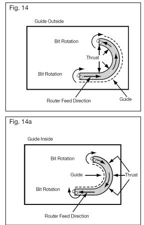
"Climb Cutting" around curves. In either case, Fig. 14 or Fig. 16a, the sideways thrust of the router cutting is always against the guide, as is proper.
