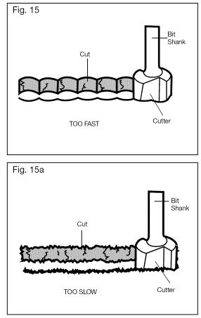
When the cutting bit is scraping instead of cutting, the router is more difficult to control as you feed it.
