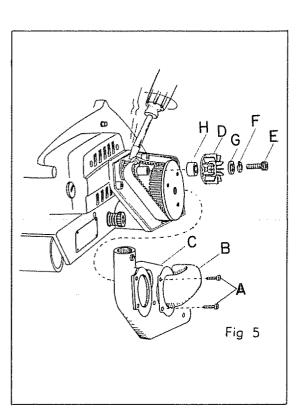
CAUTION — TO RETAIN ELECTRICAL INSULATION AND PROVIDE USER PROTECTION AS PROVIDED IN ORIGINAL DESIGN, ALL PARTS REMOVED MUST BE REASSEMBLED AND THE REPLACEMENT BELT MUST BE AN IDENTICAL REPLACEMENT PART.
