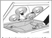
A rod swings up to support the top for cleaning underneath.
