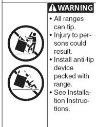
A WARNING To reduce the risk of tipping of the range, the range must be secured by properly installed anti-tip screws provided with the range. To check if the screws are installed properly, raise the lift-up cooktop and verify that the anti-tip screws are engaged. Refer to the installation instructions for proper anti-tip screw installation.
