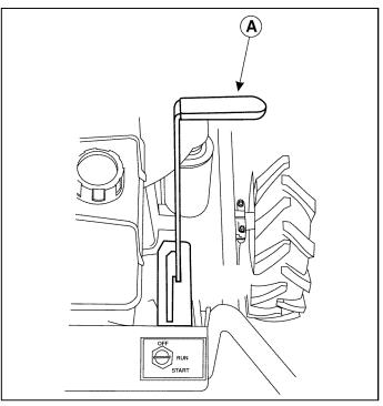
Figure 7 - PTO Engaged A. Blade Engagement Lever in engaged position.
