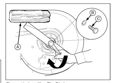
Figure 15 - Installing The Blade
