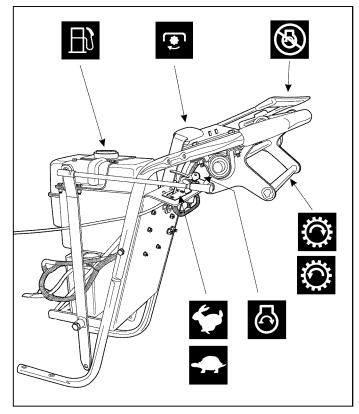
Figure 3. Brush Mower Controls
