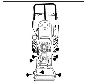
Figure 10 - Lubrication Points
