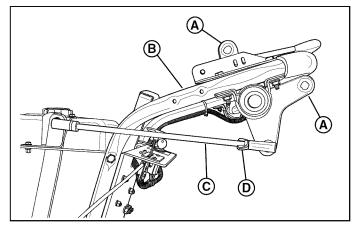
Figure 16a - Travel Controls Adjustment
