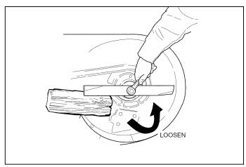
Figure 14 - Removing the Blade
