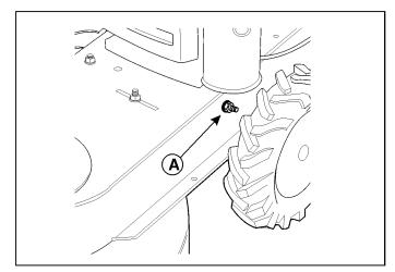
Figure 22 - Traction Drive Belt Adjustment A. Adjustment Nut
