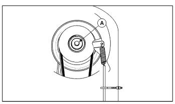
Figure 18 - Blade Spindle Brake A. Spindle Bolt
