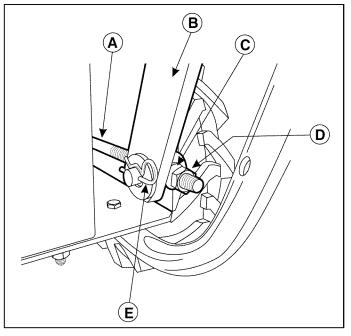
Figure 17 - Blade Clutch Adjustment
