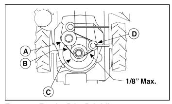
Figure 21 - Traction Drive Belt Adjustment
