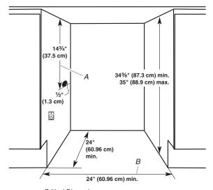
Critical Dimensions: A. 143/4" (37.5 cm) utility opening B. 24" (60.96 cm) minimum opening width
