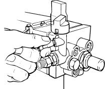
3. Press the return tube onto the brass fitting and fasten the return tube with the clamp provided.
