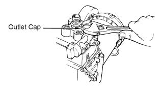
2. Leave the copper washer under the cap in place.
