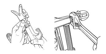
NOTE: When attaching the tip to the gun, align the tip guard as shown in the figure below, then tighten with an adjustable wrench.
