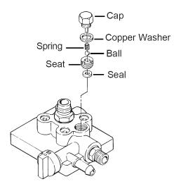
NOTE: Wear on the ball is almost impossible to detect visually. To test for a worn outlet valve assembly, turn the pressure control knob clockwise to its highest setting and run water only through the sprayer for 10 to 15 minutes without triggering the gun.
