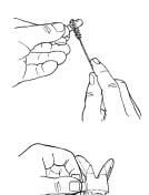
5. Attach the paint hose to the gun and tighten using two adjustable wrenches.
