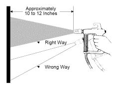
The spray gun should be triggered by turning it on and off with each stroke. This will save paint and avoid paint buildup at the end of the stroke. Do not trigger the gun during the middle of a stroke. This will result in an uneven spray and splotchy coverage.
