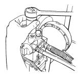
Test movement of the valve by pushing on it from the open end of the valve housing with a screwdriver or the eraser end of a pencil. It should move about 1/16 of an inch. If it does not move, it should be cleaned or replaced. NOTE: The inlet valve must be oiled after every job.
