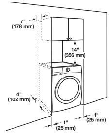
All dimensions show recommended spacing allowed, except for closet door ventilation openings which are the minimum required.
