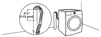
Minimum diameter for a standpipe drain: 2" (51 mm). Minimum carry-away capacity: 17 gal. (64 L) per minute. A ¹/4" (6 mm) diameter to 1" (25 mm) diameter Standpipe Adapter Kit is available (Part Number 3363920). Top of standpipe must be at least 30" (762 mm) high; install no higher than 96" (2.44 m) from bottom of washer. If you have an overhead sewer and need to pump higher than 96 inches, a sump pump and associated hardware are needed. See "Alternative Parts".
