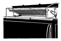
Slide a new charcoal filter into place. The filter should rest at the angle shown.
