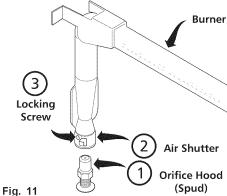
Retest the burner by repeating step "d" above. When the burner flame is a distinct blue color burning steady, the air shutter is adjusted correctly.
