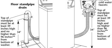
\*\*If the drain height is greater than 96 inches, a sump pump system must be used.
