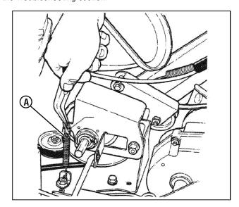
Figure 26: Replacing the drive spring
