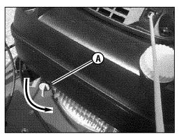
Figure 5: Fuel shut-off (Kawasaki engine only)
