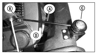
Figure 13: Installing the adapter standoff (Kawasaki engines only)
