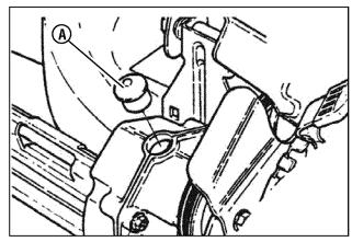
Figure 17: Removing the transmission fill plug
