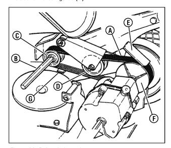
Figure 36: Poly-v belt routing
