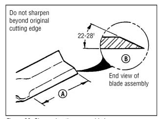
Figure 23: Sharpening the mower blade
