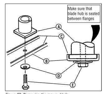
Figure 22: Removing the mower blade
