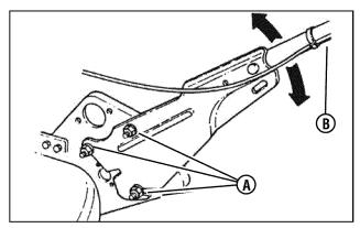
Figure 7: Adjusting the handle height
