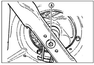
Figure 19: Tightening the blade cap screw
