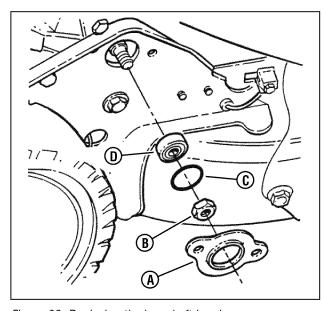
Figure 33: Replacing the hex shaft bearing
