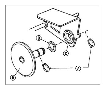
Figure 32: Replacing the driven disc
