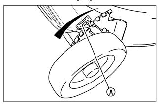
Figure 8: Adjusting cutting height
