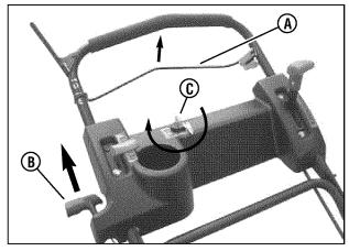
Figure 4: Starting the mower
