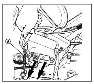
Figure 31: Removing the driven disc assembly
