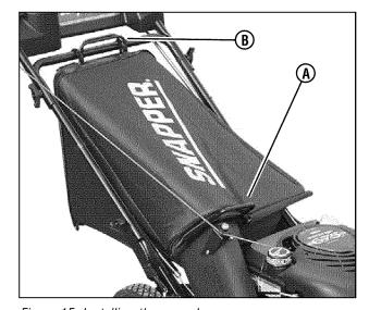
Figure 15: Installing the grass bag
