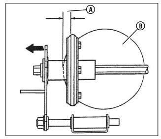
Figure 29: Proper driven disc adjustment
