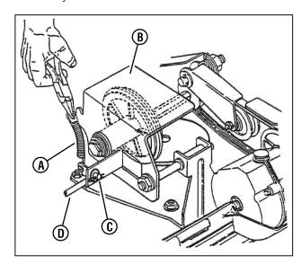
Figure 28: Adjusting the driven disc
