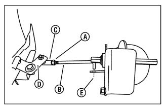
Figure 30: Adjusting the transfer rod
