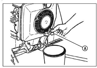
Figure 16: Draining the engine oil
