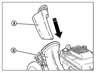
Figure 14: Installing the recycling plug
