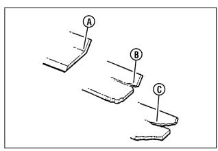
Figure 20: Standard blade wear limits
