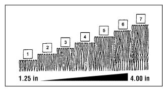
Figure 9: Cutting height settings (approximate)
