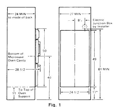
Minimum height for bottom of cutout. This places inside of microwave oven cavity 40" above floor.
