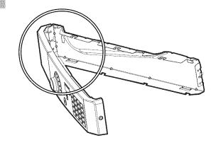
Insert the three of hooks into the holes in the frame and push it inward.
