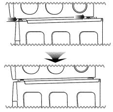
Insert the front stacking kit. Push the front stacking kit back to the stoppers of side stacking kit
