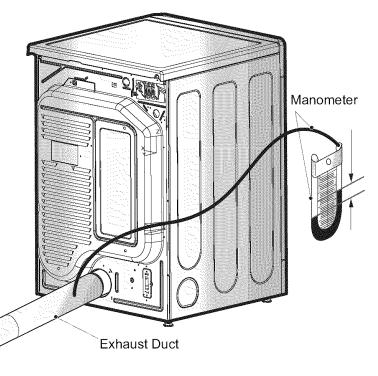
MAXIMUM STATIC PRESSURE IN WATER COLUMN
