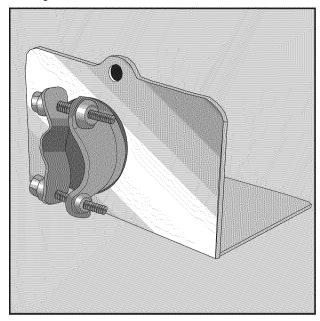
Attach the strain relief (not included) to the strain relief plate. The two screws on the back of the strain relief should be positioned as shown to prevent interferences during assembly. Tighten the strain relief lock nut to prevent the strain relief from turning.
