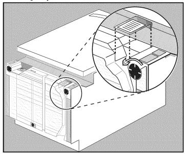
While unit is still in position as shown here, remove the junction box cover and set it aside. You will need it later.
