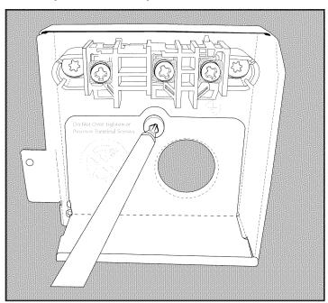
Once you remove the junction box, remove the strain relief plate located directly behind the junction box cover. **DO NOT DISCARD!.** You will re-install this later.
