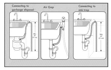
Note: Plumbing installations will vary - refer to local codes. Drain hose included is 92'' (234 cm) and can be extended to a maximum of 150'' (381 cm). Ensure a portion of the drain hose is raised at least 20'' (51 cm) above the floor.
