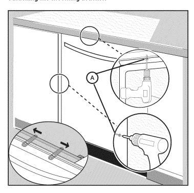
Prior to attachment, for top mount ensure that brackets are positioned as far apart as possible by sliding them within slots in direction of arrows.
