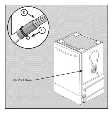
Attach drain hose (part D) to plumbing with screw clamp (part C) and tighten. Do not make any connections to the air vent hose.
