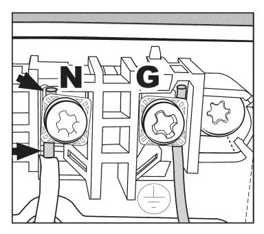
Make sure that the exposed (non-insulated) portion of each stripped wire shows above and below the terminal screw. Securely tighten the terminal screws, but **do not over-tighten** or damage may occur.
