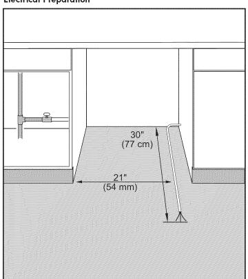
Turn power off at fuse box. Regardless of where the electrical supply cable originates, position it 21" (54 cm) from the opening's left side. Extend the cable 30" (77 cm) from the back wall.
