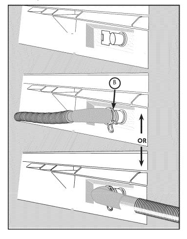
To attach the drain hose, orient it towards the direction of the sink. IMPORTANT: Route hose towards sink PRIOR to connection. DO NOT rotate the hose after attaching it to the dishwasher. This would cause it to crimp. Attach the drain hose elbow to the back of the unit with the **included** spring clamp.
