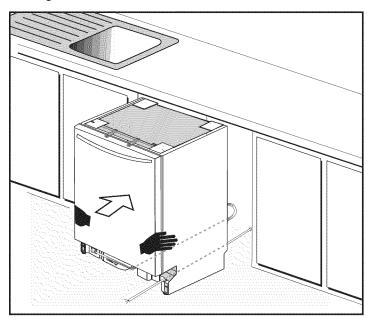
Place hands where pictured to push into place. Guide the water line and drain hose toward the sink, and electric line through the proper channel. Units are typically positioned so that the door is flush with cabinet door and drawer fronts. For optimal noise reduction, ensure side strips are in contact with cabinet.
