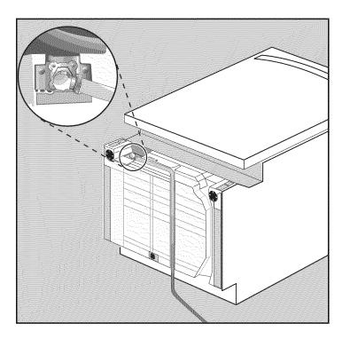
Attach hot water line to 90° elbow and route water line through channel as shown (stainless steel braided hose and PEX installations only - for copper consult a plumber). Regardless of where the electrical supply cable originates, position it 21" (54 cm) from the opening's left side. Extend the cable 30" (77 cm) from the back wall. Use tools recommended by the hot line manufacturer.
