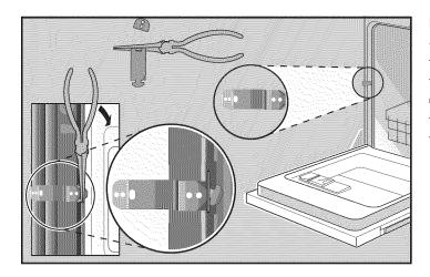
If your dishwasher has the pre-attached mounting brackets and the countertop is stone, use pliers to rotate the bracket flanges so that you are able to remove brackets from the top. Grasp bracket with pliers at perforation and bend until rounded end breaks free. Discard end. Slip brackets through side slots. Using pliers, bend bracket flanges so that the brackets will not slip through slots. Do not attach yet.
