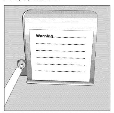
Replace junction box cover. Make sure the cover is seated behind the front lip of the strain relief plate. Attach the cover with the screw (part F) from the installation kit.
