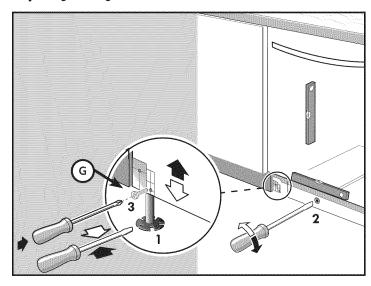
NOTE: If the dishwasher is not level, it may not operate properly and could cause leaks.
