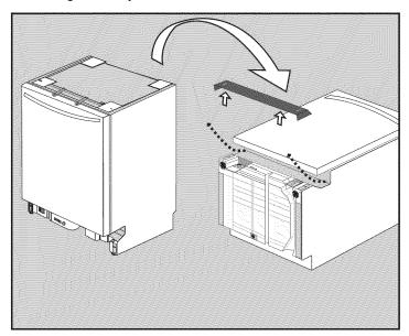
Gently rest the unit on its back. Remove the toe panel. Set the toe panel aside. It will be installed later.
