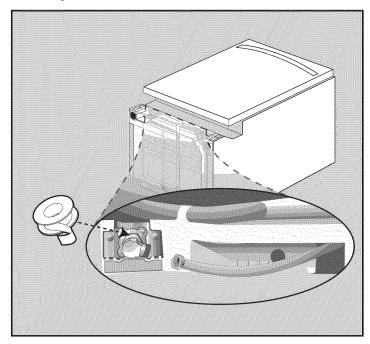
NOTE: The 90° elbow fitting is not supplied with the dishwasher and must be purchased separately (see "Materials Needed" section).
