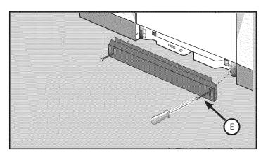
Attach the metal toe panel with screws (Part E) so it is flush with the floor. Your installation is now complete.
