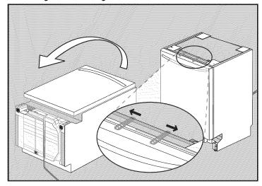
Flip unit back upright, ensuring water line remains in appropriate channel and is not pinched. If your dishwasher has the pre-attached mounting brackets as shown and you have a wooden undercounter, ensure that brackets are positioned as far apart as possible by sliding them in direction of arrows. Do not attach to countertop yet.
