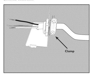
Pass wires through strain relief and plate. Leave 3 to 4 inches of insulated wire extending through the strain relief plate. Tighten clamp around wires, oriented as shown. Bending the electrical cable as shown will ease installation of the strain relief plate.
