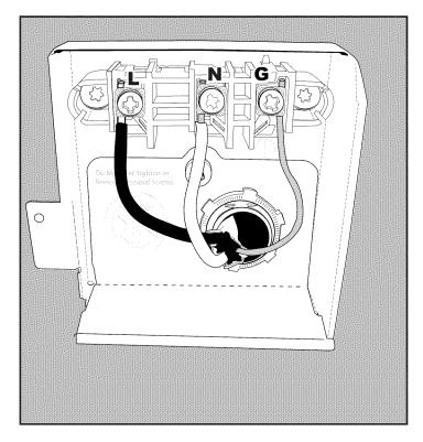
**Note:** Do not loosen or remove terminal screws! Damage may occur. Bend the wires so the exposed leads can reach the appropriate contacts. Insert the black (hot) wire into the left opening on the terminal strip marked "L", the white (neutral) wire in the middle opening of the terminal strip marked "N", and the bare copper or green (ground) wire into the right opening of the terminal strip marked "G".
