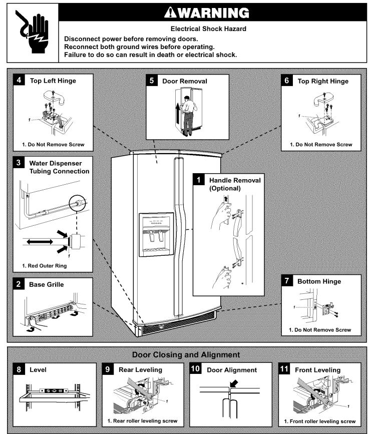
**NOTE:** It may only be necessary to remove either the door handle or the doors to get your product through the doorway of your residence. Measure the door opening to determine whether to remove the refrigerator handles or the doors.
