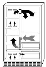
Do not block any of these vents with food such as soda, cereal, bread, etc. If the vents are blocked, airflow will be prevented and the temperature controls will not function properly.
