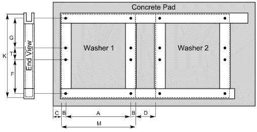
Dimension chart for foundation base, anchor bolt placement, and elevated concrete pad
