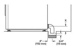
Minimum Waste Channel Measurements
