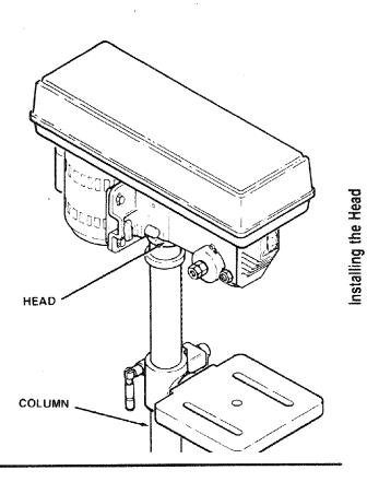
3. Using a 4mm Hex "L" wrench tighten the head lock set screws on the right side of the head.
