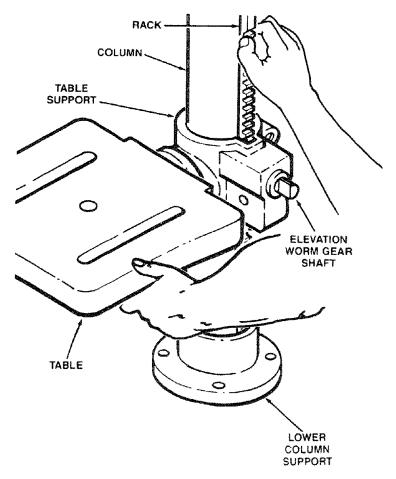
4. Replace column collar and position it bevel side down over rack. Tighten set screw in collar with 3mm HEX "L" wrench. To let the rack slide when the table is swung to the left or right around the column, the collar must sit loosely over rack and should not be angled on the column. Only tighten set screw enough to keep collar in place, otherwise the collar may be broken due to excess pressure.
