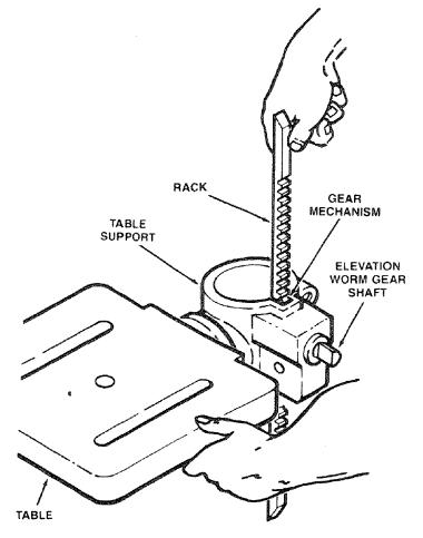
3. While holding rack and table support in an engaged position slide both down over column. Slide rack down column until rack is positioned against lower column support.
