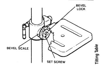
WARNING: TO AVOID INJURY FROM SPINNING WORK OR TOOL BREAKAGE, ALWAYS CLAMP WORKPIECE AND BACKUP MATERIAL SECURELY TO TABLE BEFORE OPERATING DRILL PRESS WITH THE TABLE TILTED.
