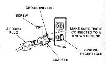
**NOTE:** The adapter illustrated is for use only if you already have a properly grounded 2-prong receptacle. Adapter is not allowed in Canada by the Canadian Electrical Code.
