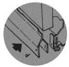
Turn on water and check for leaks at fitting. Reinstall the 2 access panels on the lower front of the dishwasher.
