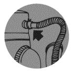
Turn electricity on. Run a cycle to check for leaks at both the hot water and drain connections. When water and drain connections are working, cancel cycle.
