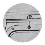
Connect the dishwasher to the drain using the silver clamp provided.
