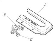
A. Anti-tip bracket B. Plastic anchors (2) C. #10 x 1" screws (2)
