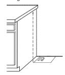
If cabinet opening is wider than that specified in the "Location Requirements" section, adjust template so range will be centered in cabinet opening.
