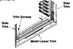
b. Using three trim screws provided, secure the bottom trim to the bottom edge of the cabinet.
